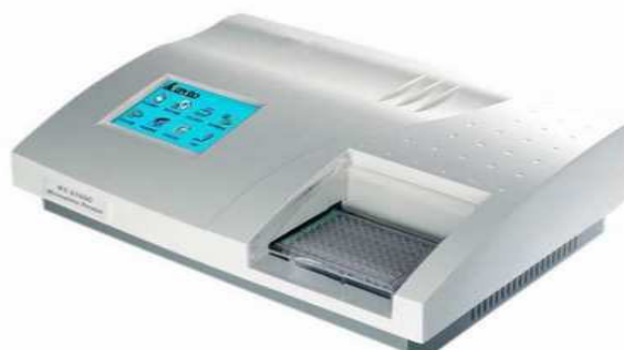
Figure 2 shows the equipment where the AFM1 quantification was performed at a wavelength of 450 nm.
