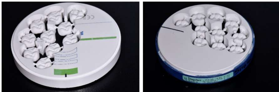
Figure 2. Restorations on CAD-CAM disks of zirconia dioxide before sintering.
