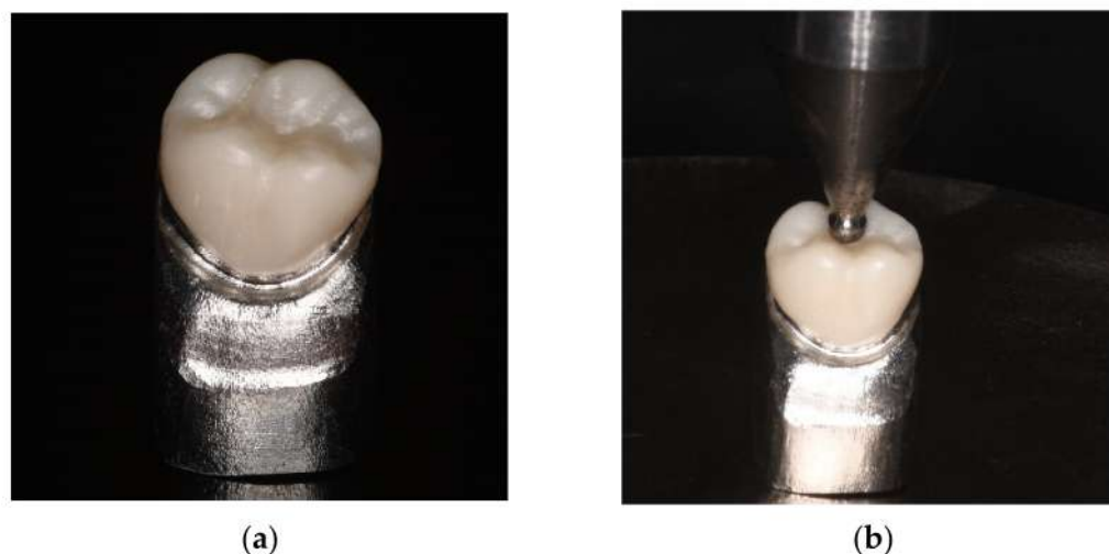
Figure 3. (a) Master die in cast metal. (b) Load of the punch in tempered steel on the sample seated in the cast metal die.
