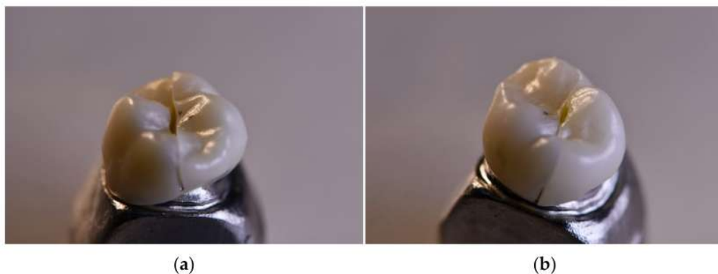
Figure 6. Images of the fracture surfaces of the different materials studied: (a) CDS; (b) ZGX.
