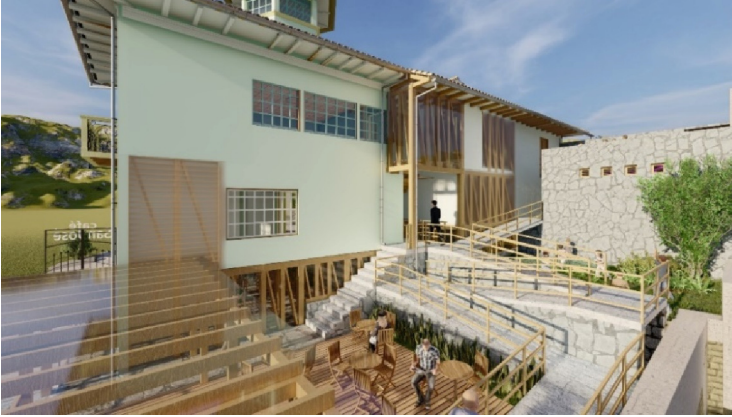
Fig. 7. Intervention proposal, reinterpretation of bahareque to replace severely damaged walls. Source: Own (2020)
