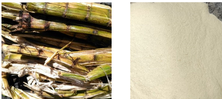
Figure 1. Untreated and ground sugarcane bagasse.
