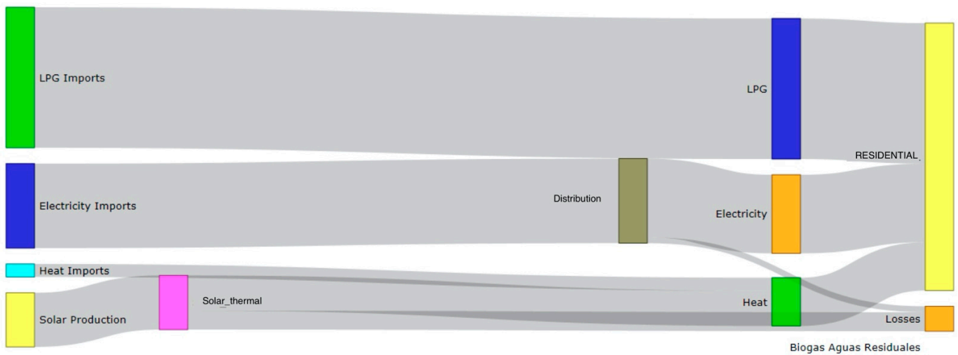
Figure 7. Scenario 2. Sankey diagram for 2030, residential sector (The figure shows the electricity losses given by the local distribution company. In addition, the losses of conversion of solar energy to heat are displayed. Losses due to the commercialization and distribution of LPG have not been included).
