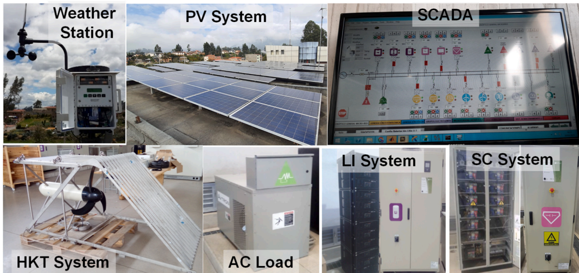
Fig. 7. Equipment used for power smoothing tests in the microgrid laboratory of the University of Cuenca.
