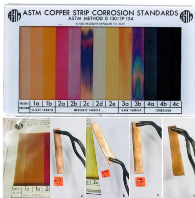
Figure 2. (a) Corrosion to copper caused by biodiesel obtained with 0.5% NaOH; (b) corrosion to copper caused by biodiesel obtained with 1% NaOH; (c) corrosion to copper caused by biodiesel obtained with 0.5% KOH; (d) corrosion to copper caused by biodiesel obtained with 1% KOH.
