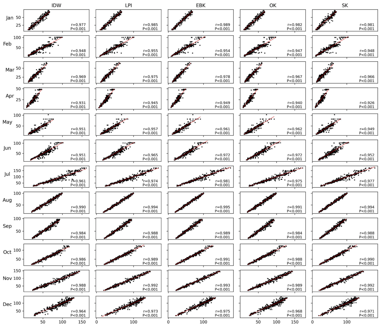
Fig. 4. Scatterplots of measured (y-axis) vs. predicted (x-axis) tropospheric NO 2 columns from IDW, LPI, EBK, OK and SK. The trendline, the Pearson coefficient (r) between the measured and estimated, and P value are shown.
