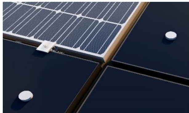
Figure 5. Integration of PV panels and dummy modules in the roof for ventilated roof configuration (own elaboration)
