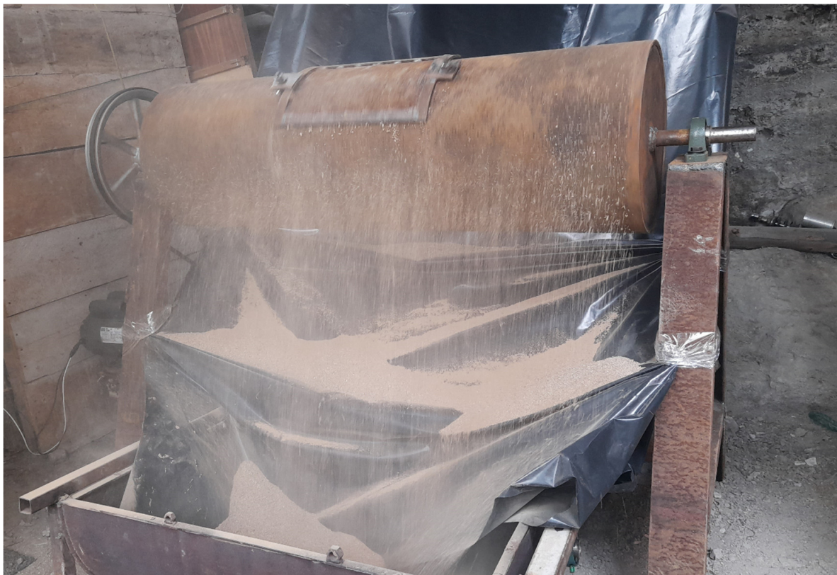
Figure 2. Sifting cylinder manufactured for the crushing and sifting of the earth.
