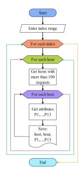
Fig. 4. Flowchart for obtaining the attributes to generate the DNS fingerprints.
