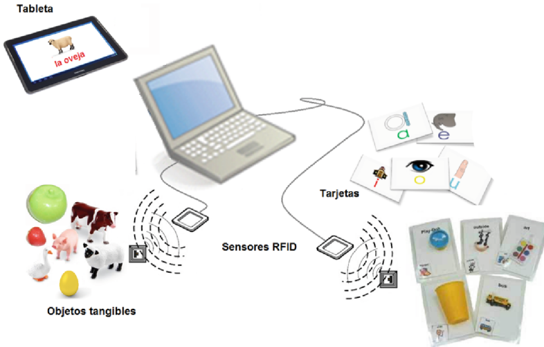
Fig. 2. RFID technology to build tangible pictograms
