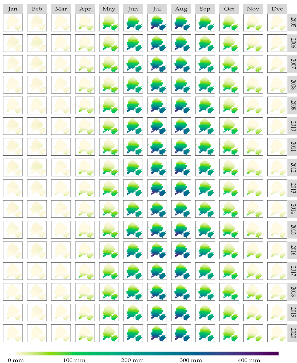
Figure 5. Spatial-seasonal distribution of rainfall forecast with the polynomial model, sample from the years 2005 to 2020.
