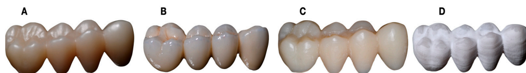
Figure 1. Four-unit FDP structures used for this investigation. (A) ZR O 2 (KATANA, Zirconia STML), (B) PFM, (C) PMMA (Telio CAD) and (D) 3DPP (SprintRay ONX).
