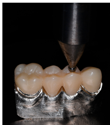
Figure 3. Application of compressive tests on FDPs' structures, performed on a universal test machine.
