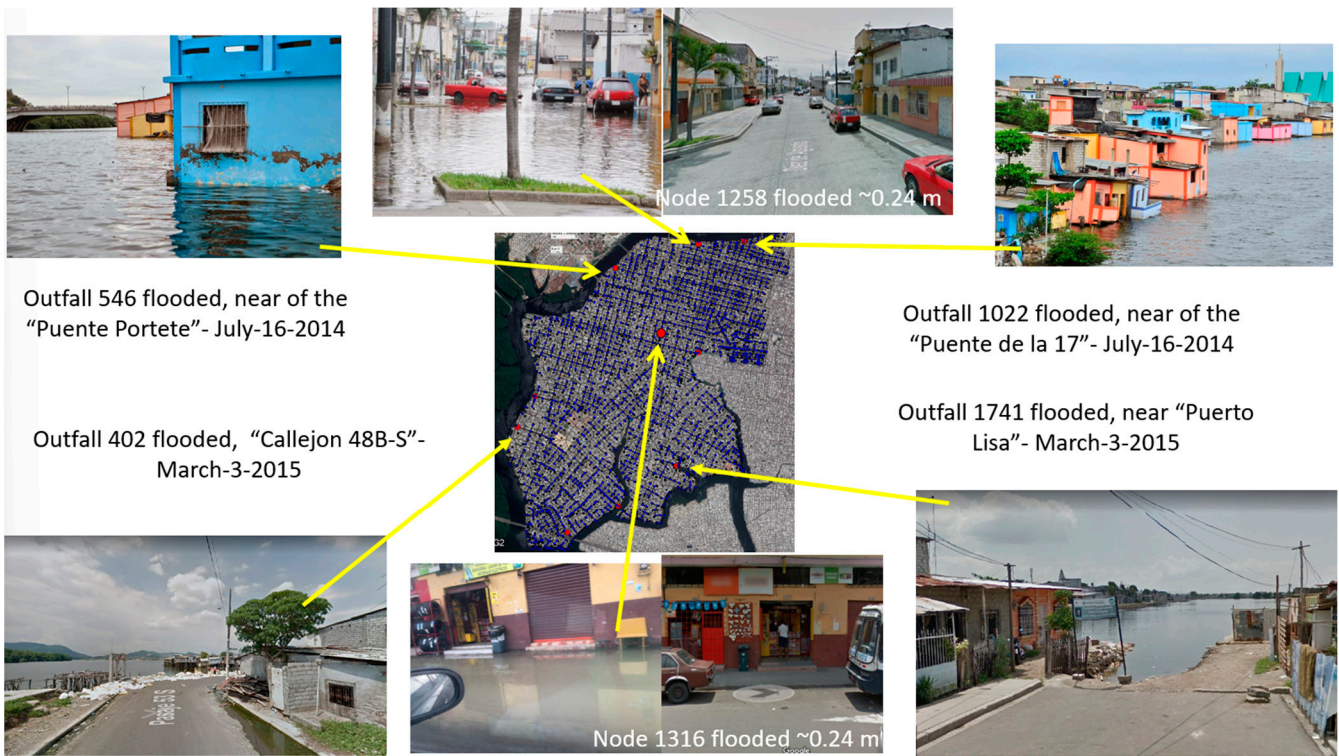
Figure A2. Calibration of boundary conditions with levels checked with photographs. Photos taken by the authors.
