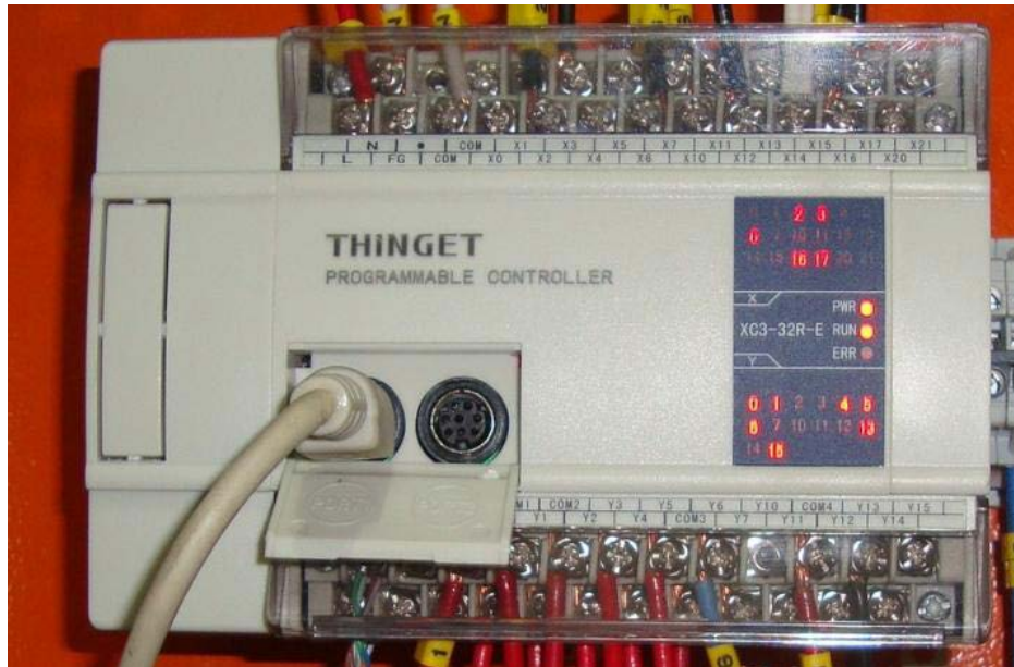
Figura 1.5. PLC Thinget XC3-32R-E.
