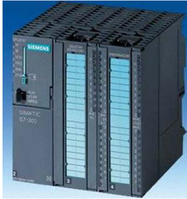
FIG.15 a PLC Siemens S7-300 19
