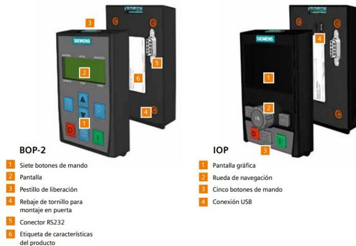
**FIG.20** “Basic Operator Panel 2” y el “Intelligent Operator Panel” <sup>26</sup>
