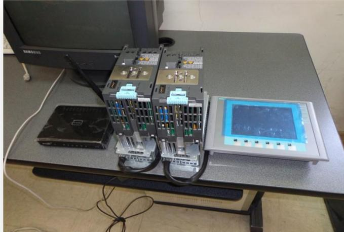
**FIG.125** HMI KTP600, DRIVE G120, Router TP-Link 600
