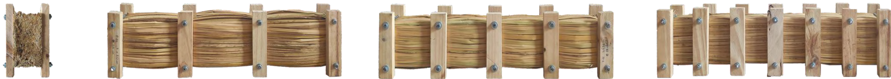
Figura 142. Prototipo final P.03 (18 x 20 @ 20, 15, 10 cm)
