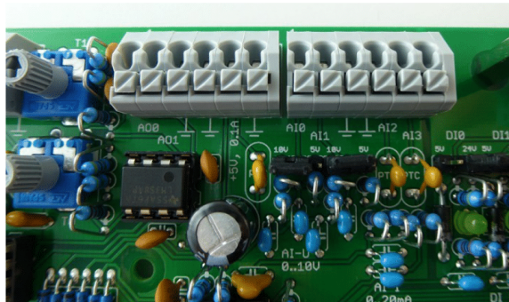
Figure 25: Connector blocks - analog in- and outputs
