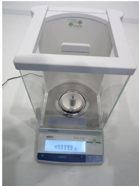
Figura 10: Balanza digital Mettler Toledo Monobloc modelo AB204-S.
