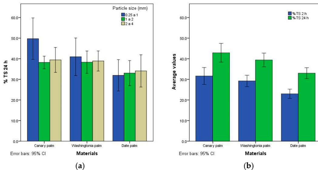
**Figure 4.** (a) Average TS values after 24 h of water immersion according to the palm species and particle size (b) Average TS values after 2 and 24 h according to palm species.
