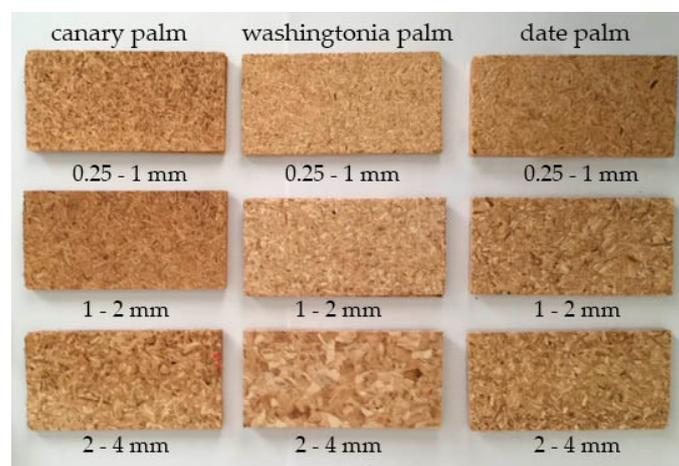
Figure 2. Particleboards made with rachises of different palm species.
