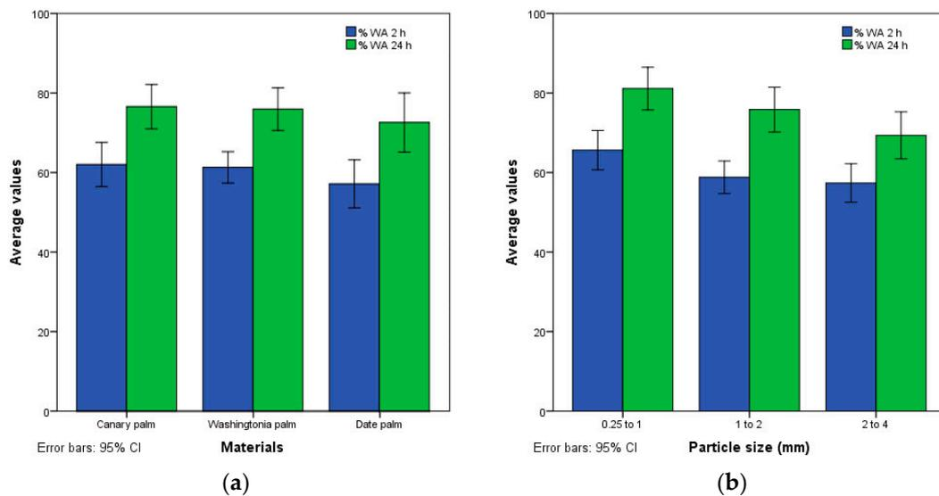
**Figure 5.** (a) Average WA values after 2 and 24 h of water immersion according to palm species. (b) Average WA values after 2 and 24 h of water immersion according to particle size.
