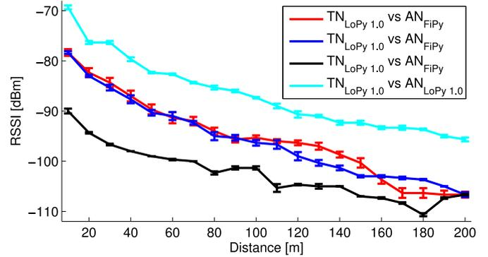
Fig. 9. The characteristic curve of the return link for the 90 m × 90 m scenario with  $BW = 500$  kHz,  $SF = 12$  y  $P_{TX} = 5$  dBm.
