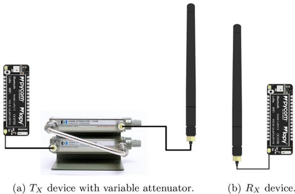
Fig. 4. Dynamic range tests of RSSI sensitivity.
