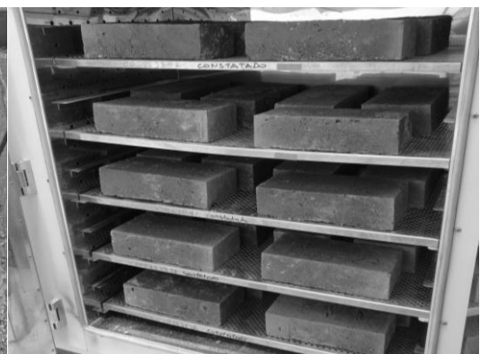
PERALTA JORGE, 2017, Secado Artificial de ladrillo. [Imagen 10]
