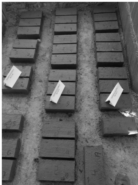
PERALTA JORGE, 2017, Secado natural de ladrillo . [Imagen 37]
