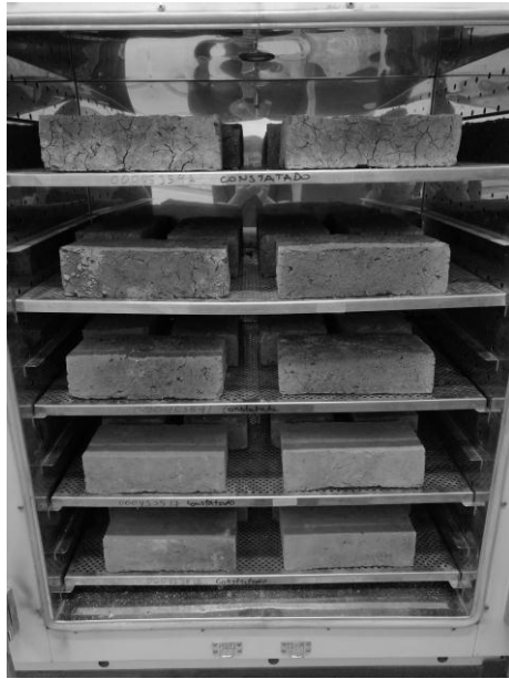
PERALTA JORGE, 2017, Secado artificial de ladrillo. [Imagen 39]
