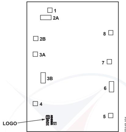
Figure 53. Bond Pad Diagram
