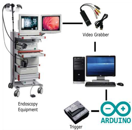
Figure 2. Diagram describing the connection between the host gastroenterology equipment and the developed hardware
