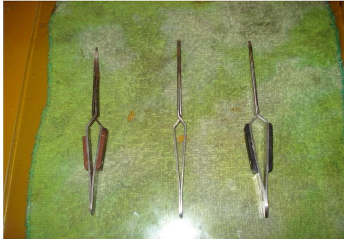
**Figura 58. PINZA PARA SOLDAR**
