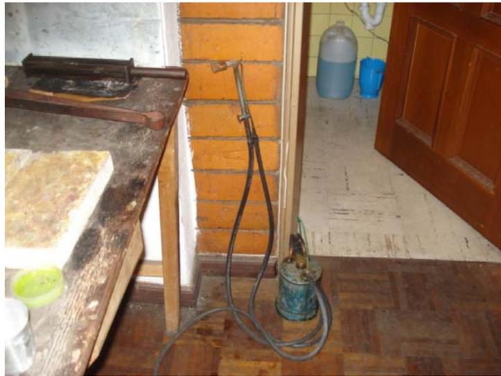
**Figura 3. SOPLETE DE SOLDAR**
