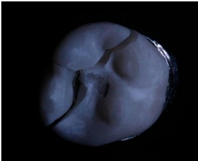
Figure 4. Fractured 3DPPb Crown.
