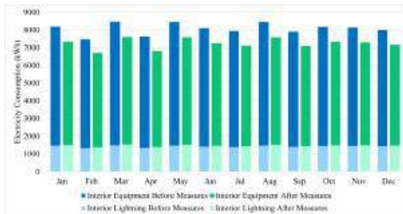
Fig. 4. Monthly overview of electricity consumption before and after measures.
