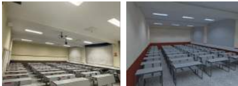
Fig. 3. Comparison between a real image (left) of the A-005 classroom and its simulation in DIALUX® (right).
