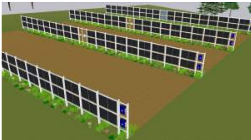
Fig. 1: Vertical bifacial facility for agrivoltaics.
