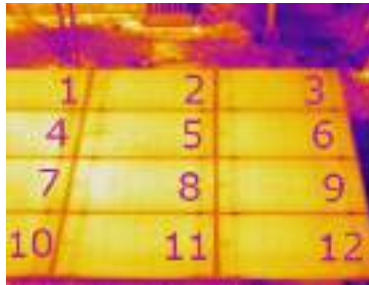
Fig. 1. Segmentation of the solar array used by the system. Module 2 serves as a reference for the calculation of temperature gradients.
