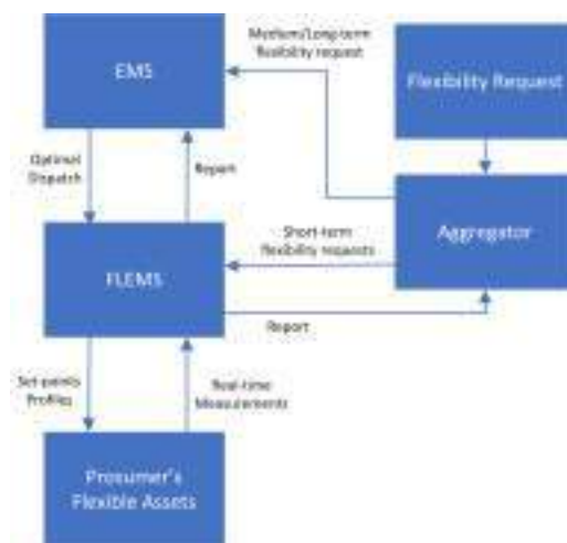
Fig. 1. Control Scheme of Power System with Distributed Resources
