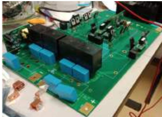
Fig. 5. DC/DC photovoltaic converter in development.
