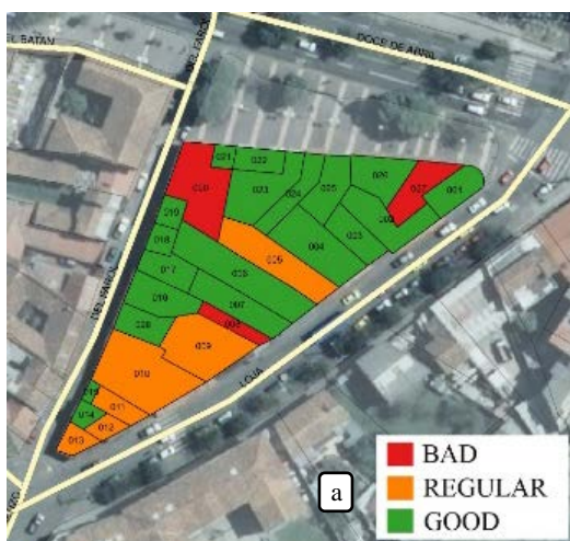
Figure 2a: The condition of the buildings in the Diagnosis phase, before the Campaign (2012). Source: vlirCPM project.
