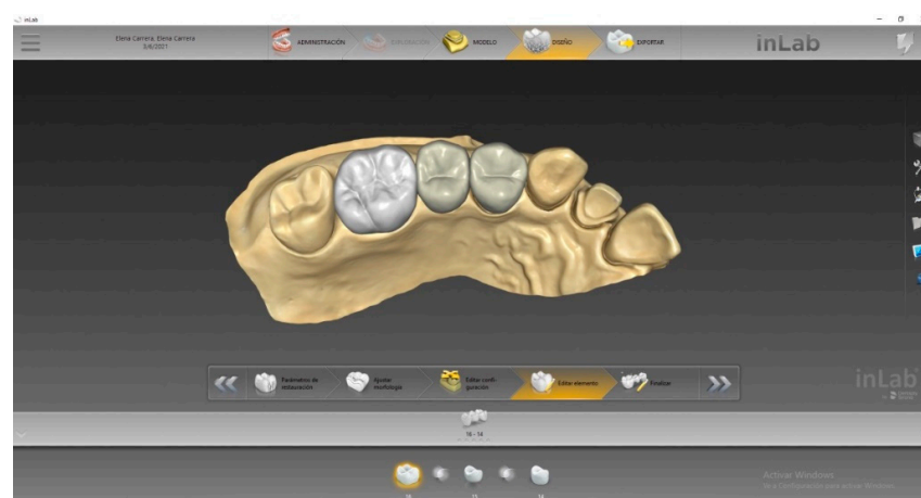
Figure 2. Design of a three-unit fixed dental prosthesis (FDP) using biogeneric modality.
