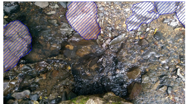
Fig. 3 Schematic for the determination of the ratio between the projected area occupied by large size particles and total plan area. The hatched areas represent large, immobile particles. (ESC 1:20).
