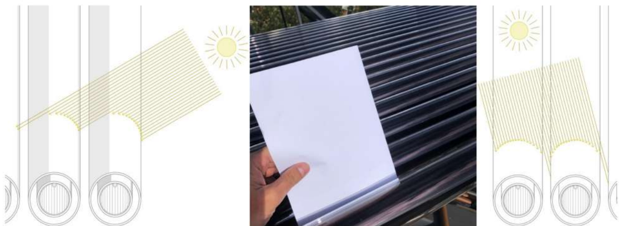
Figure 4. Diagrams showing solar incidence on the vacuum tubes and irradiance blocking at 8 a.m. and at 1 p.m. The photograph shows the solar incidence on the equinox at 8 a.m. in south-facing ETCs.
