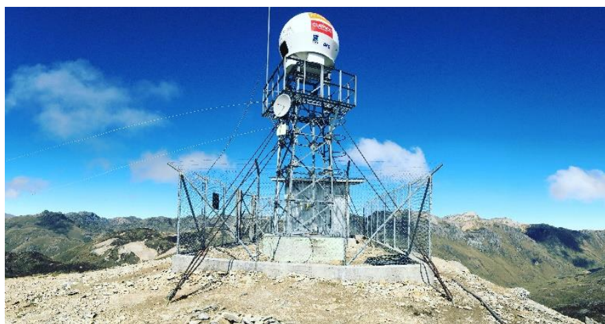
Figure 2. X-band radar station: Radar CAXX Rainscanner-RS120 on Paragüillas peak (4450 m a.s.l.).
