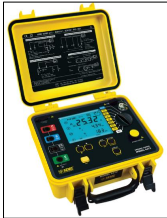
Figura 3. 3 Ground Tester AEMC Model 6472 [3].
