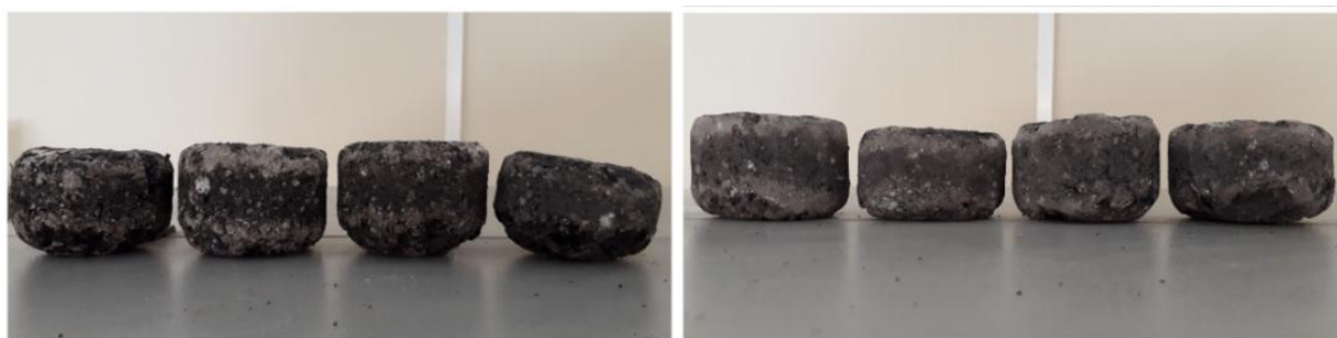
Fig. 5. Abrasion results comparison, for 6% PET (left) vs. 0% PET (right)
