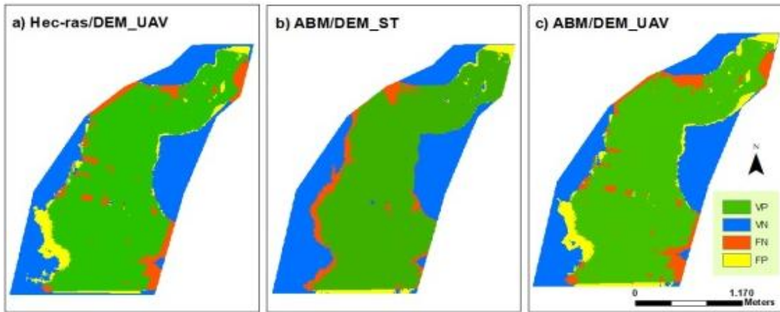
Fig 8 Validation maps. a) Generated with the Hec-ras and DEM_UAV model. b) Model ABM and DEM_ST. c) Model ABM and DEM_UAV.
