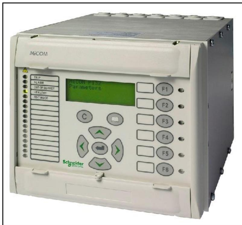
**Figura 2.9** Relé diferencial digital Schneider. [14]
