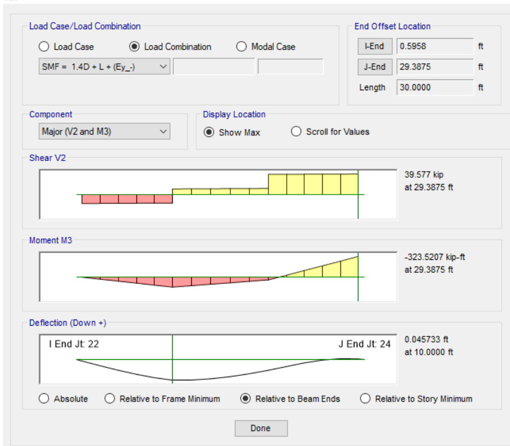
Diagram for Beam B22 at Story STORY5 (W18X65)
