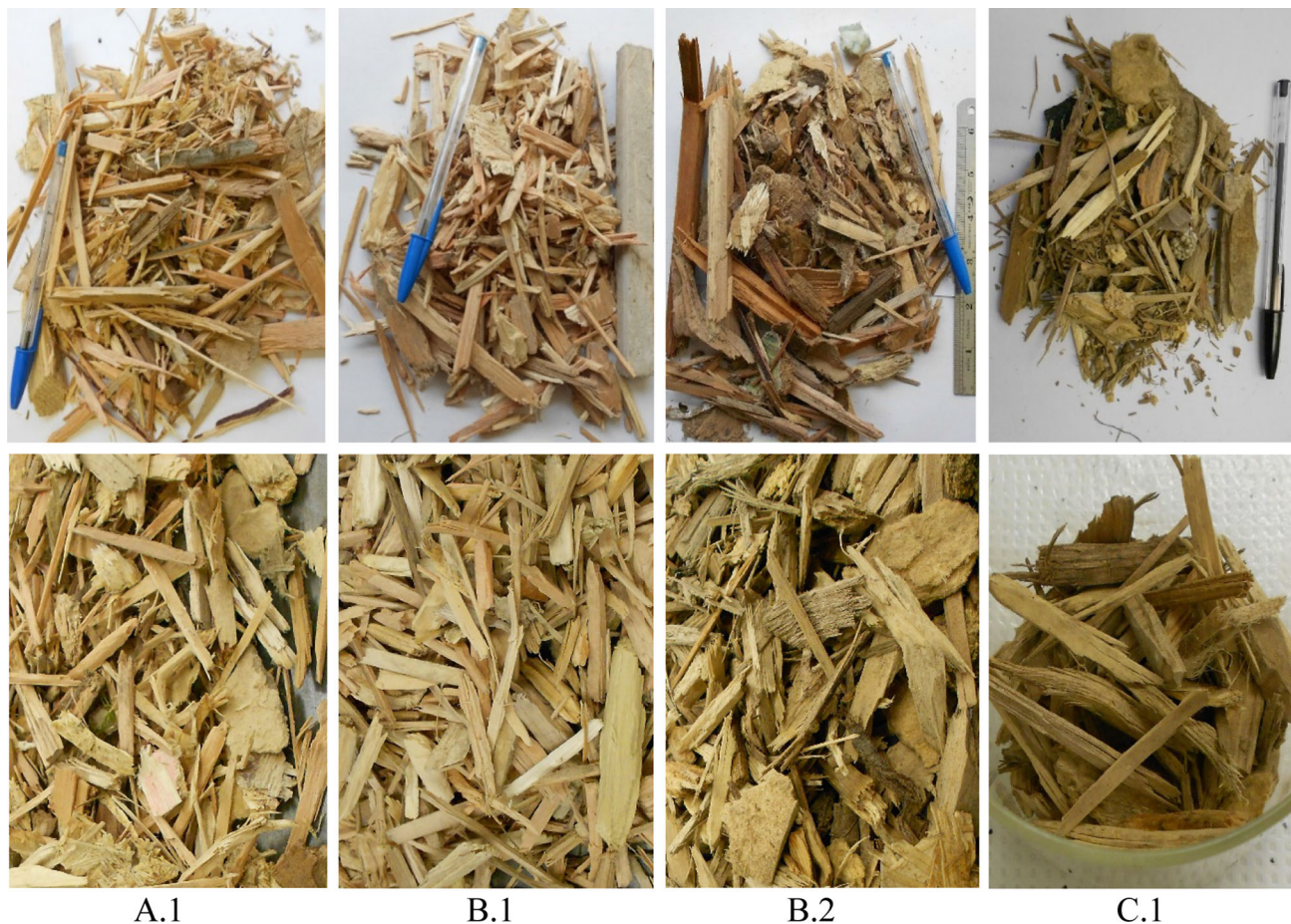
Fig. 1 Pictures of the WWR samples as received ( upper row ) and as used for the SPORL process ( lower row ). The “as received” samples were constituted by mixes of splinters, chips, slivers, wood
