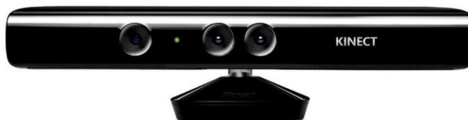
Figura 2-5 Sensor Kinect
