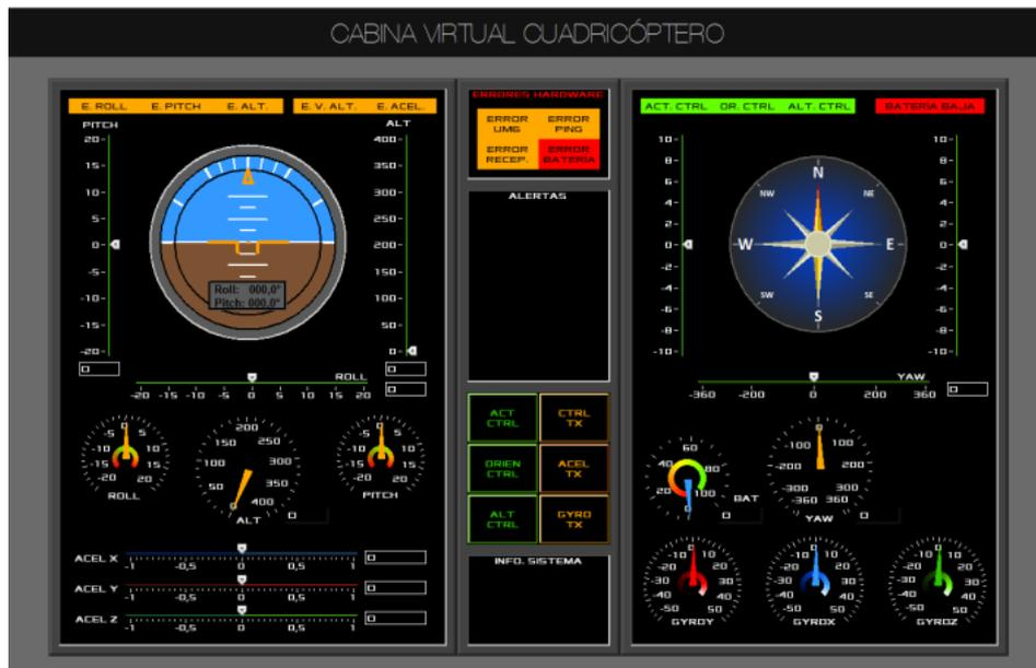
Figure 6. Virtual cockpit on the HMI.
